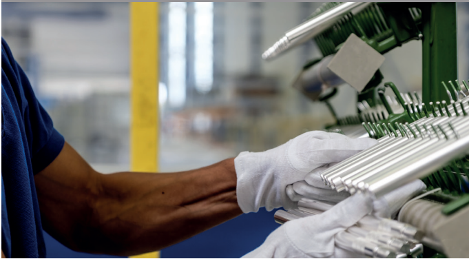
Silver plating on a dynamic rotating rack
