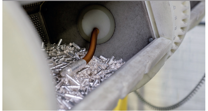
Silver barrel plating by barrel plating
