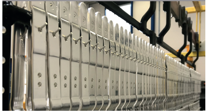
Silver plating on a static rack
