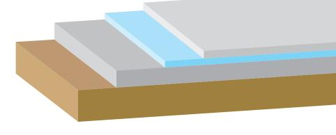
This image shows a cross-section (not to scale) of a typical Zn-Ni coating. The three layers of coating consist of a layer of Zn-Ni alloy, covered by a layer of chromate, with a topcoat or sealant on top.
