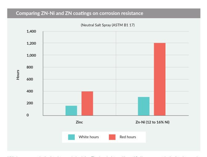
White hours represent the time it took to corrode the plating. (Zinc degrades into a white rust.) Red hours represent the time it took to corrode the substrate, wich usually forms red rust.
