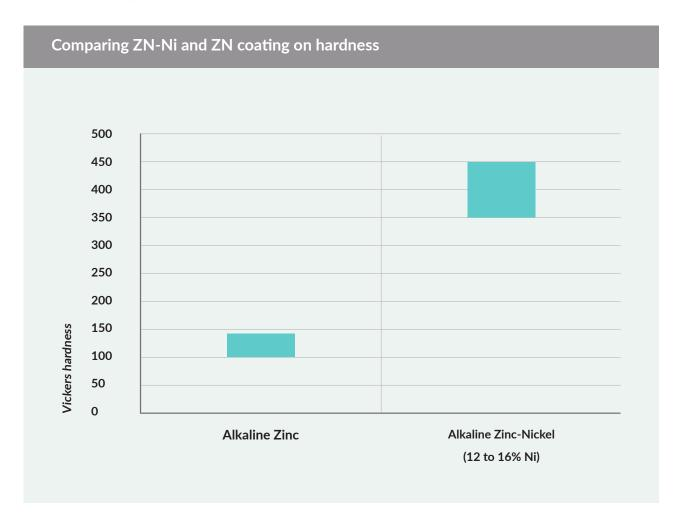
These laboratory tests reveal that Zn-Ni coating offers a unique set of qualities not found in other electroplated or traditionally applied coatings. Experience has shown that these qualities play a significant part in extending the life cycle of equipment and structures.
